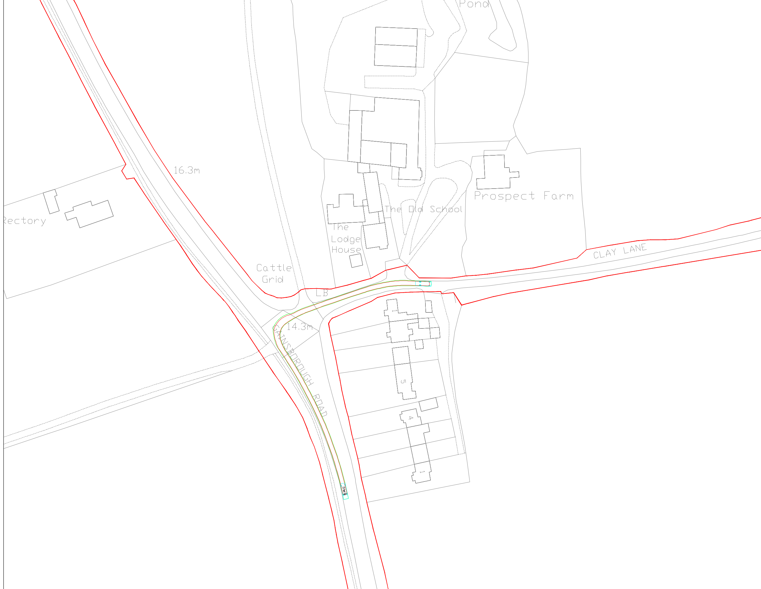
7.5t PANEL VAN VEHICLE MANOUVRE, HEADING NORTH ON GAINSBOROUGH ROAD A156 TURNING RIGHT INTO CLAY LANE HEADING EAST - SCALE 1:1000
